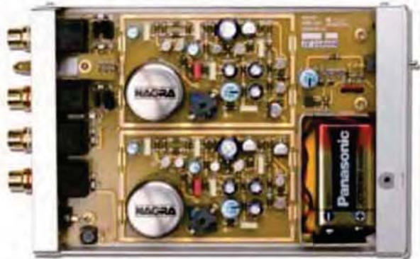
Inside the BPS—two transformers, one 9V battery.
